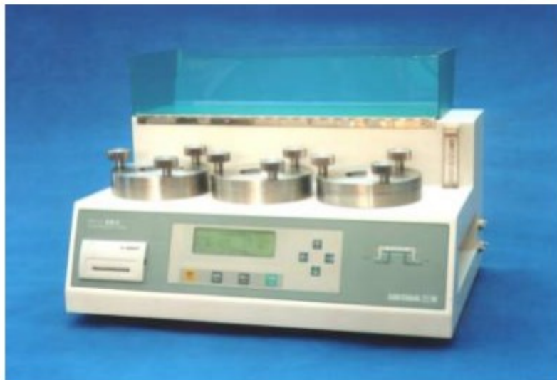
Fig.3. TOY-C1 Package/Film Oxygen Permeability Tester (fitted with the film sample)
